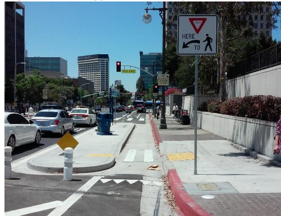
Figure 4-2 - Type II Floating Bus Bulb
