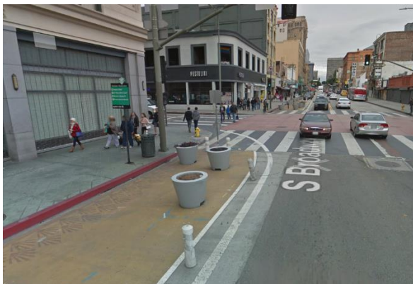
Figure 2-9 - Example of an Interim Curb Extension
