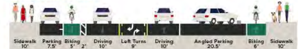
Option 1: Angled parking on north side of street with protected bike lane (westbound), conventional bike lane (eastbound)
