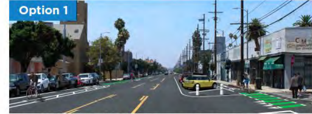
Angled parking on north side of street with protected bike lane (westbound) and standard bike lane with safety buffer (eastbound).
